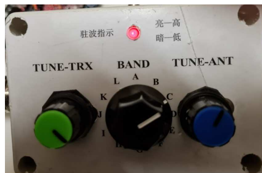
Figure 23 – Showing a match of 1:1.3 on 15m dipole at 40m – Dim LED
