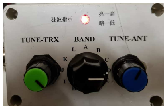
Figure 24 – Inductor deliberately changed – SWR way off – Bright LED
