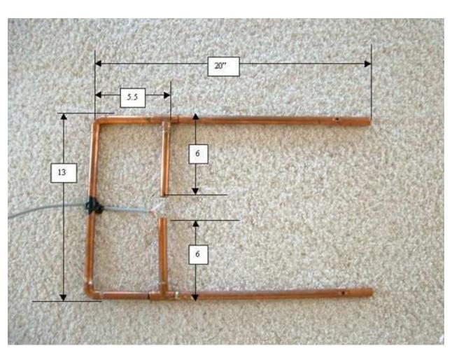
In 2003 I built one because if its novelty, plus I needed a repeater antenna for the the basement. I wanted to monitor our local 146.97 repeater while building in the basement shop. It worked well in that applicatiion. I hung it from a plastic pipe and had no problem using the repeater which was 2 miles distant, on 200mw!!!
