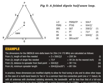
beam. I measured this to be about 240kHz with a centre frequency of 14.175MHz - a very acceptable figure for such a small beam. Those who regularly operate CW in the lower reaches of the band allocations, will find that only minor length adjustments are required at the open end. Setting the desired resonant frequency is extremely simple.
