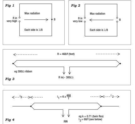
thus a half-wavelength long. The loop can be any shape, from square (with each side  $\lambda/8$ ) to circular (of radius  $\lambda/4\pi$ ). In the case of the square loop, there are two possibilities – the closed loop, as in **Fig 1**, or the open loop, as in **Fig 2**, in which the side opposite the feed-point is *open* at its centre.
