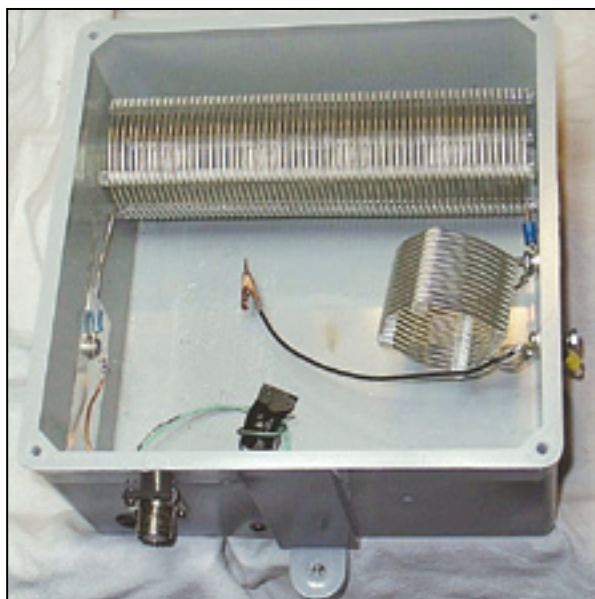
Figure 1 — The split inductor mounted in the NEMA enclosure. Alternatives are to use a larger box and keep the inductor intact or use the toroid wound inductor specified in Part 1.
